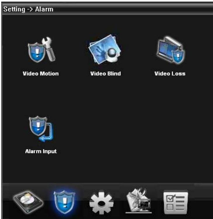
Alarm activation configuration(motion detect,video blind,video loss and alarm in),see below picture.
